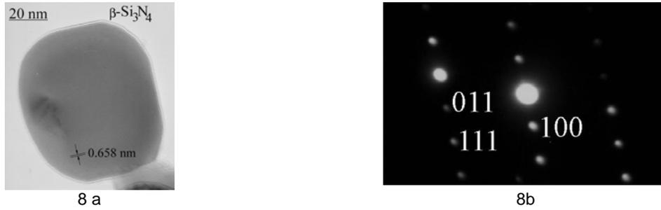
Fig. 8. (a) TEM image of a fragment of a  $\beta\text{-Si}_3\text{N}_4$  particle of the sample after 1773 K vacuum heating; (b) corresponding diffraction pattern.
